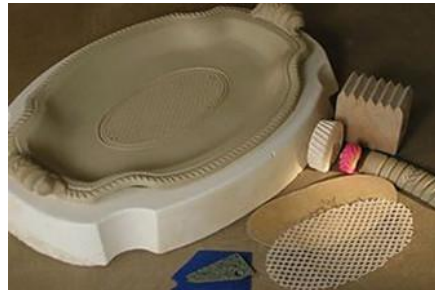
Slump molds allow you to shape the rim and/or add handles.
