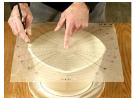
Using a needle tool to mark through the disk.
