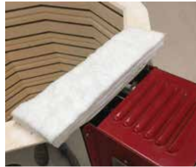
Proper placement of the ceramic fiber blanket lid prop on an electric kiln shields the control box from excessive heat while venting combustion gases.
